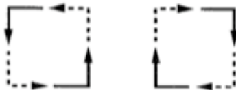
FIG. 3. The four turns allowed by the xy routing algorithm.
