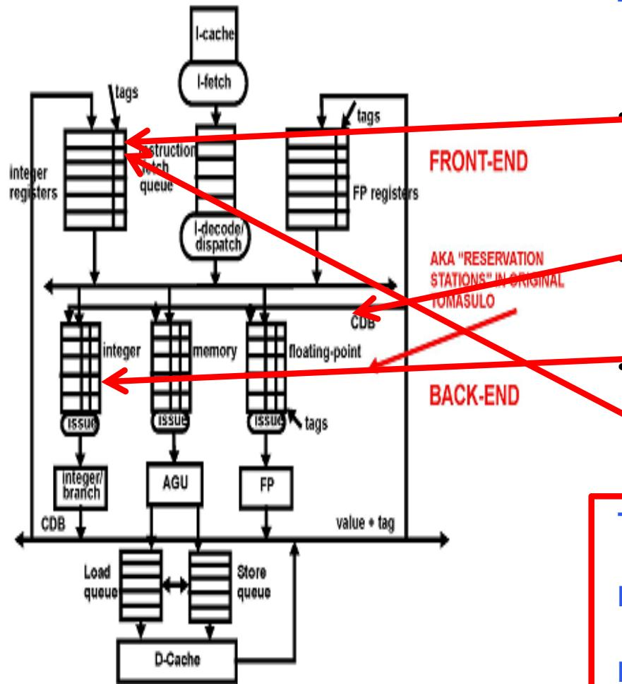
The output register is assigned a TAG (the Q entry number where instruction is dispatched)
