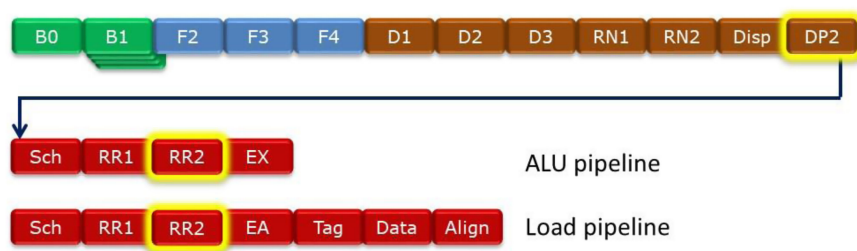
Figure 2. M3 core pipeline, with stages added to M3 highlighted.
