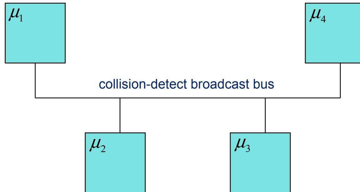
Broadcast serial bus, dual wire (resistor terminated), 1 Mbit/s
