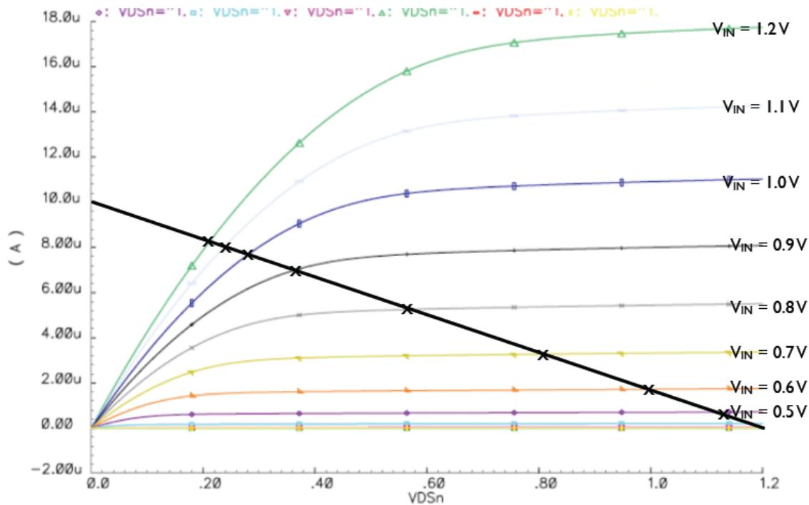
b) Where the load line intersects one of the current curves the point for the input voltage that corresponds to that input voltage. The points are marked in with crosses in the voltage diagram above. Above each point is the corresponding  $V_{IN}$  (that is  $V_{GS}$ ) value. The corresponding  $V_{OUT}$  vs  $V_{IN}$  diagram looks like this.
