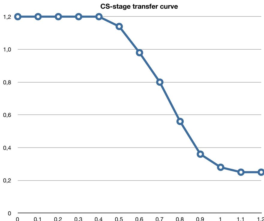
c) We can get an estimate from drawing the line in curve, or since we have so few points we can use the approximation between the two data points at  $V_{IN} = 0.7$  and  $0.8$  that gives us  $0.55-0.8 / 0.8-0.7 = -2.5$
