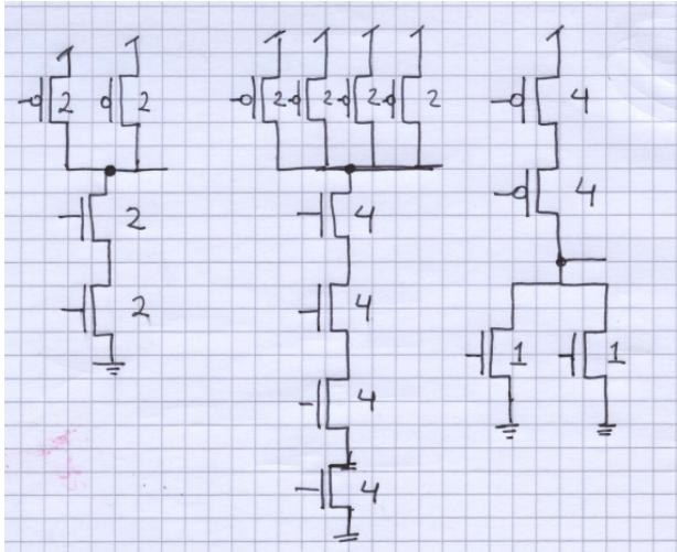
An inverter with the pMOS transistor twice as wide as the nMOS transistor is assumed to have the parasitics  $p_{inv}$ .
