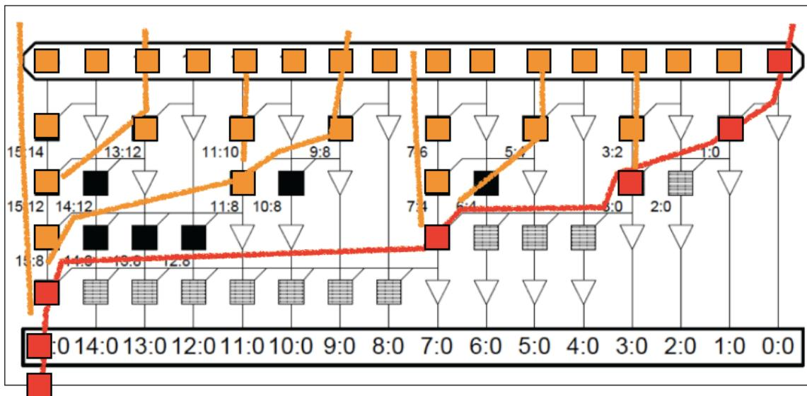
If all the red and orange cells above are implemented with cells from the fast library, bit 15 should be generated in around  $\frac{3}{4}$  of the time for the slower library.
