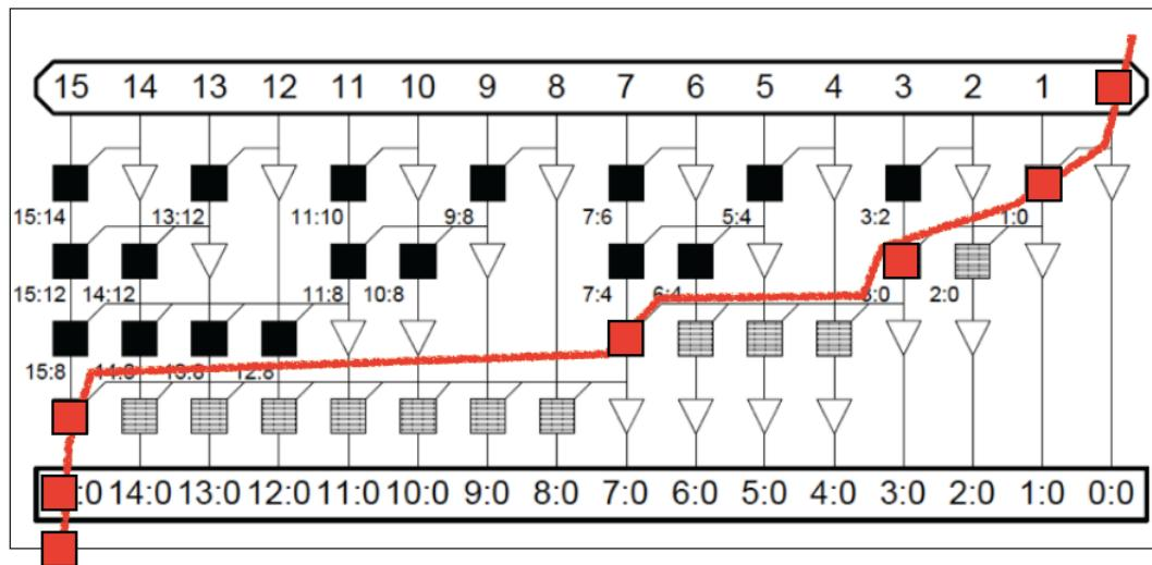
This is the path we want to speed up by using the faster library for the seven red cells. The critical path has 4 AOI cells in the tree. However, there are many additional paths with 4 AOI cells that lead to the bit15 output. Since the constant part is dominating all these paths have to also be implemented in the fast library. The figure below shows these paths and all their cells in orange:
