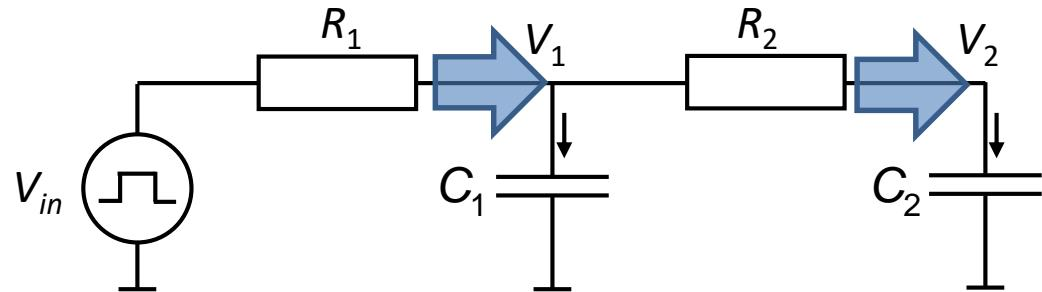
Each resistance is multiplied by its downstream capacitance!
