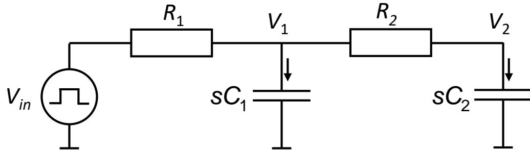
$$H(s) = \frac{1}{R_1 R_2 C_1 C_2 s^2 + (R_1(C_1 + C_2) + R_2 C_2)s + 1}$$
