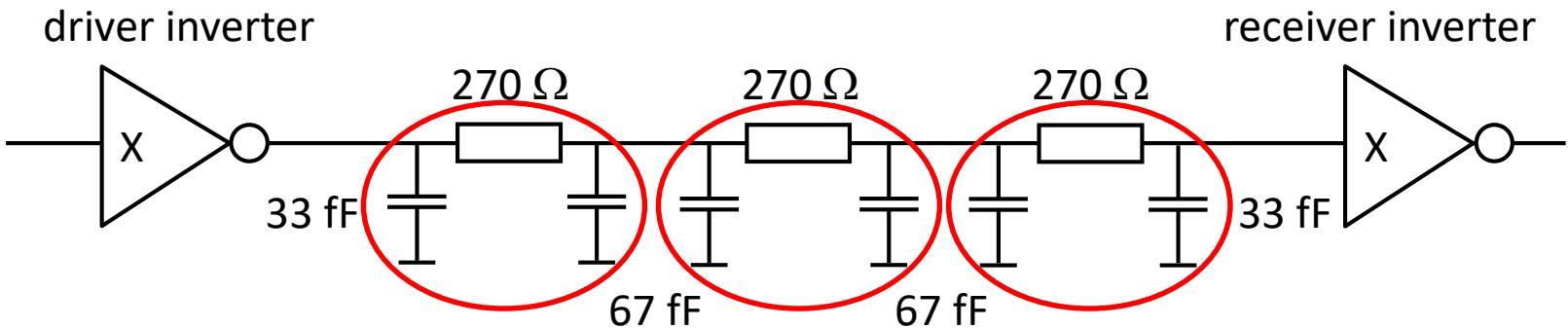
The given parameters yield a wire resistance of  $800 \Omega$  and a wire cap is  $200 \text{ fF}$ . Wire resistance is distributed along the wire which must be modeled by segments. In Spice circuit simulations a 3-segment  $\pi$ -model is accurate to within 3%. However, for simple analytical estimate: use single segment  $\pi$ -model.
