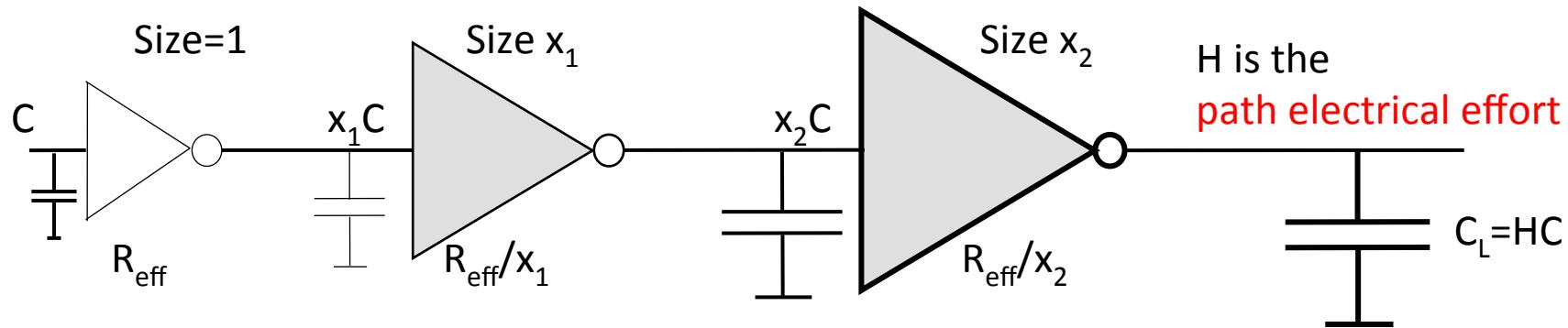
With two intermediate buffer inverters we obtain a normalized delay relative to tau:
