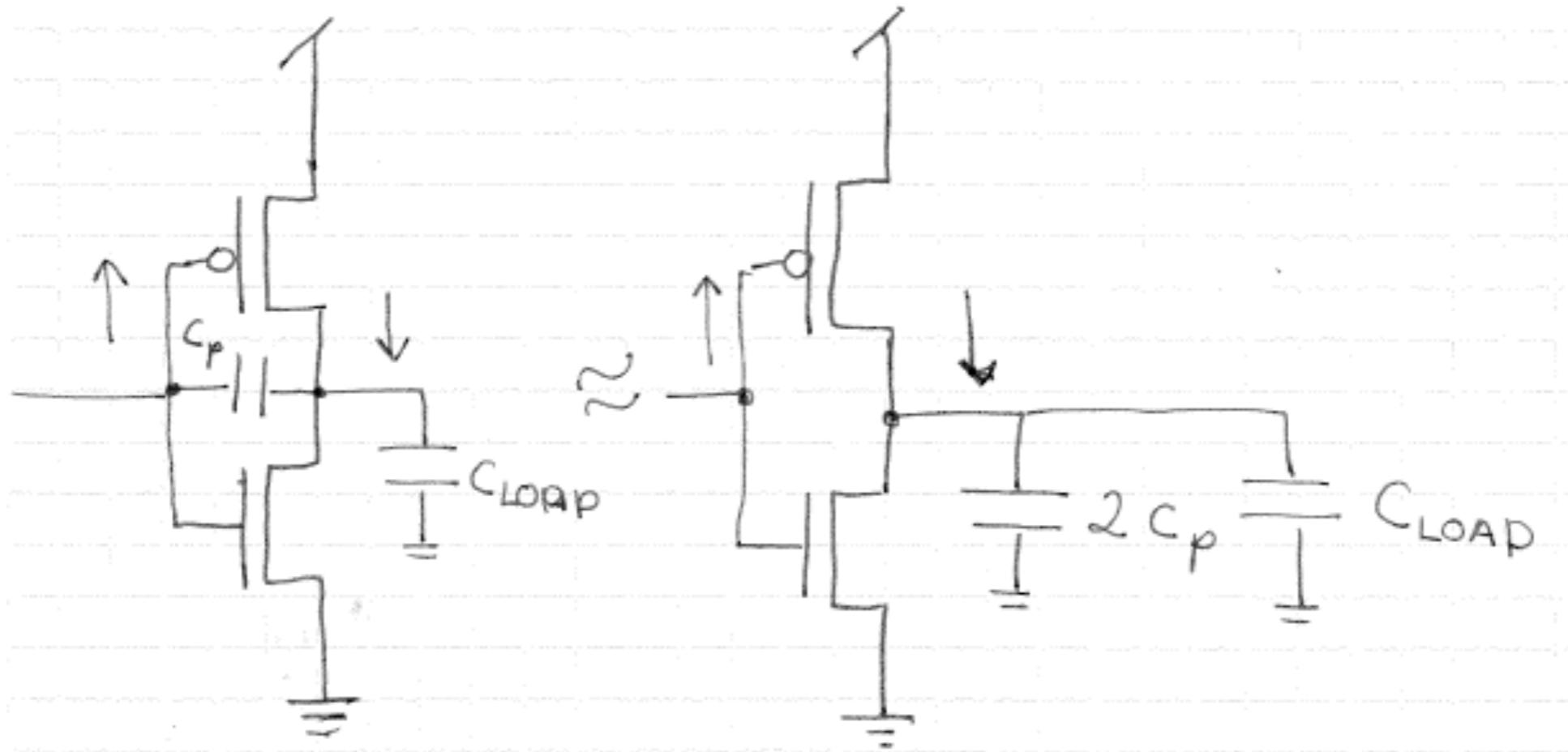
When inverter is driven by voltage source which can deliver infinite current this effect does not show.
