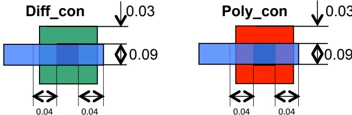
For minimum width metal lines at least 0.04 enclosure is required on two opposite sides (bottom measures).
