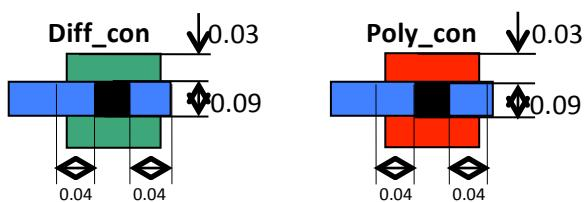
For minimum width metal lines at least 0.04 enclosure is required on two opposite sides (bottom measures).
