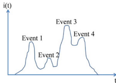
Fig. 2. Dynamic current is associated with the switching times and power draw of each gate.
