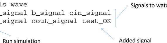
The only signal to watch in the test bench is really `test_OK` but it is practical to keep the rest of the signals for debugging
