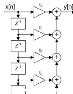
We can conclude that the impulse response has the same values as the coefficients in our FIR filter so we can use the inverse fourier transform to design our filter
