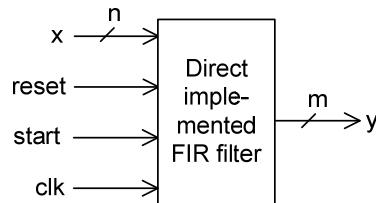
In this lab assignment we leave out the sampling of the signal and just use a start signal to trigger the calculation of a new output sample.
