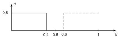
Observe that we have only specified the amplitude behaviour. We want a filter with zero phase. Such a filter can not be realized in real time but we can get linear phase which is just a delay of the signal
