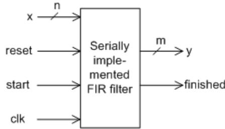
Here we need a clock signal to shift in the bits and a signal to indicate when the calculation is done
