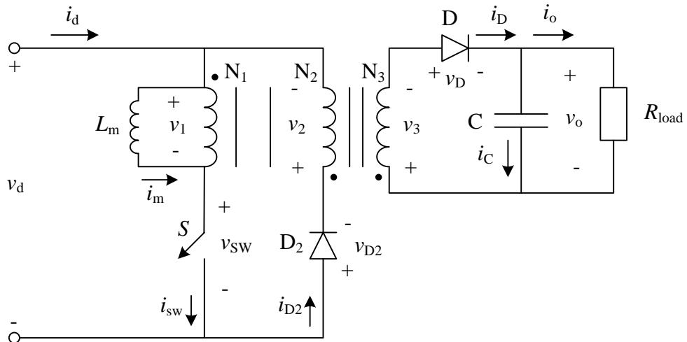
For DCM, Derive the voltage transfer ratio  $V_o/V_d$  in terms of the load resistance  $R_{load}$ , switching frequency ( $f_{sw}$ ) transformer inductance ( $L_m$ ) and duty ratio ( $D$ ).
