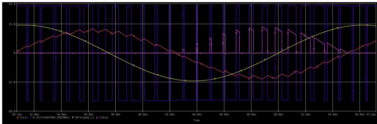
With an increase in load inductance, both the output current and current ripple are lower. The current waveform now has a THD of 4,5%, compared to 5% before.
