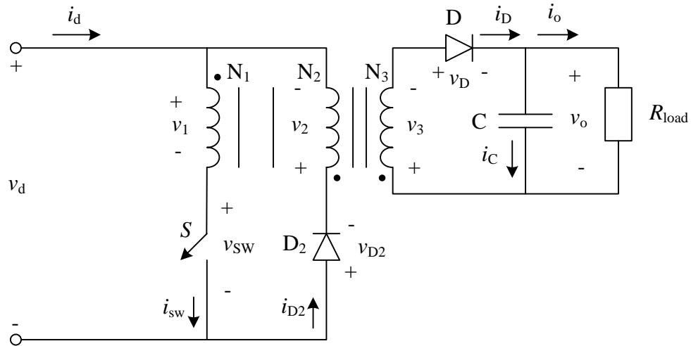
When and how does the winding  $N_2$  and diode  $D_2$  become operational to limit the output voltage?
