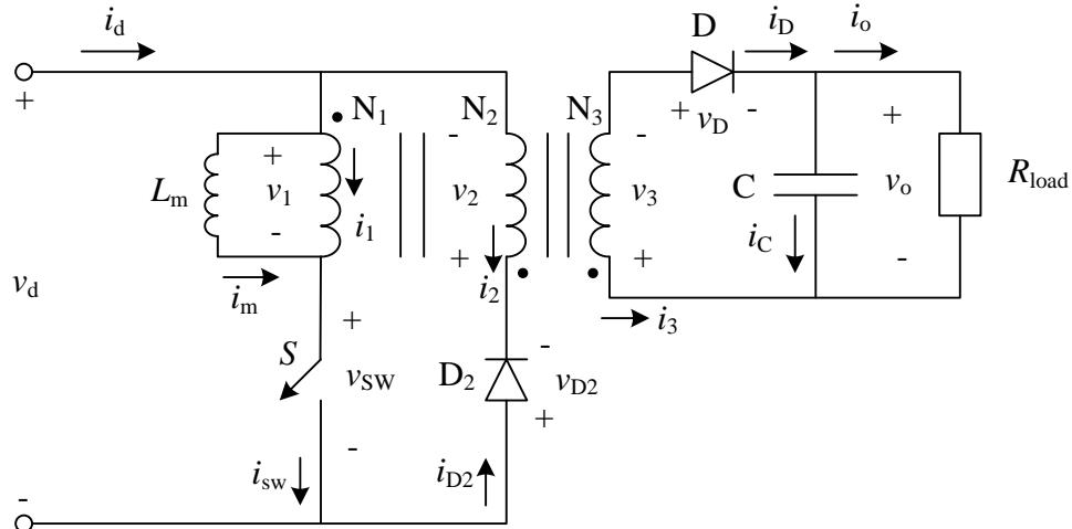
Because of the ideal transformer assumption and the three windings share the same magnetic core, the voltage ratios are derived as
