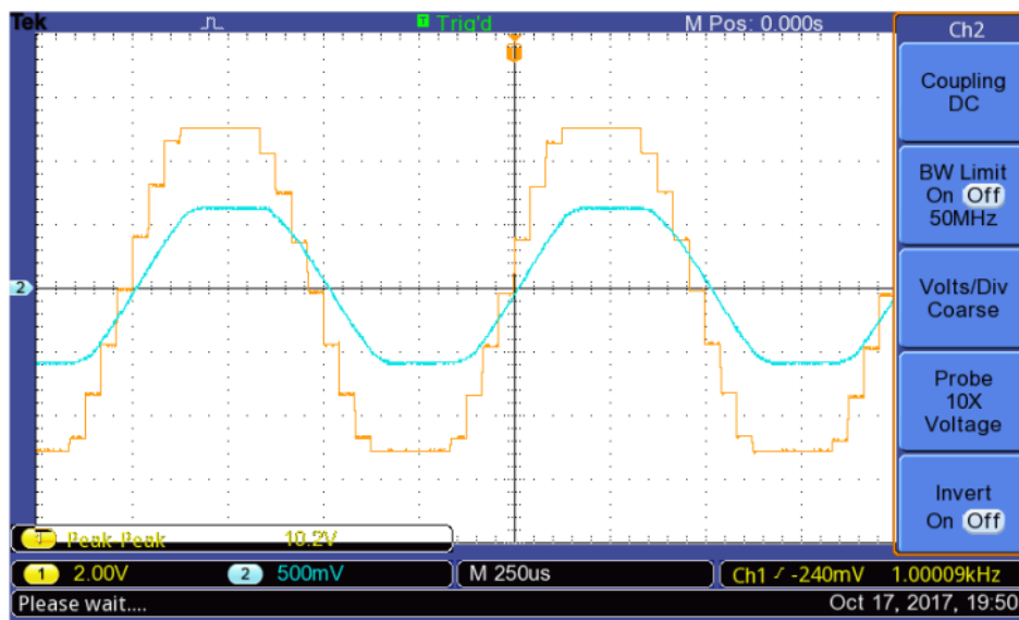
Figure 19: Noticeable clipping on the receiver. V_{DA} in Yellow, V_{amp2} in Blue
