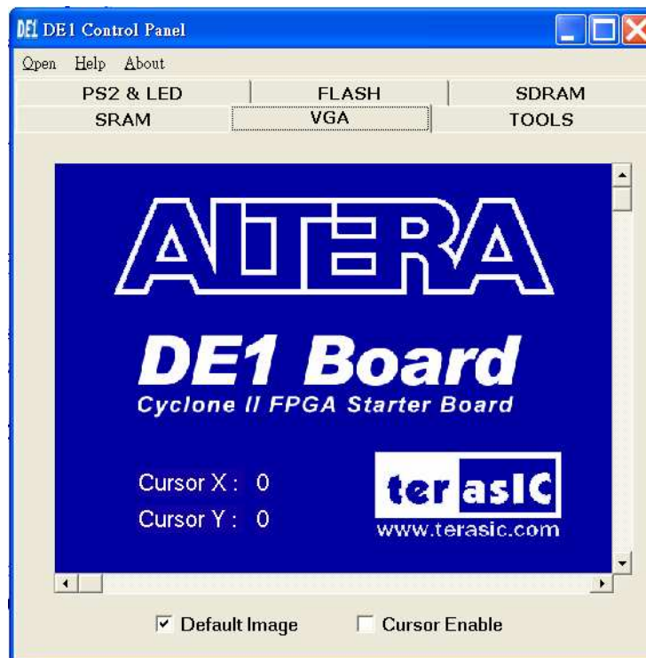
Figure 3.9. Displayed image and the cursor controlled by the scroll bars
