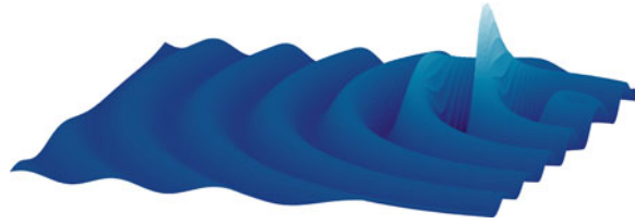
Fig. 1.4 Water ripples created in a pond by a small rock. Although the water particles move vertically, the wave expands horizontally while carrying away the kinetic energy of the falling rock. Eventually, the energy is dissipated in the pond and the wave dies out
